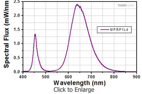
Broadband LED Spectra Scaled to Min Power
