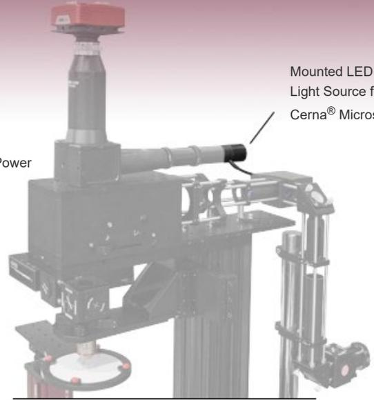
Mounted LED used as a Light Source for a DIY Cerna® Microscope
