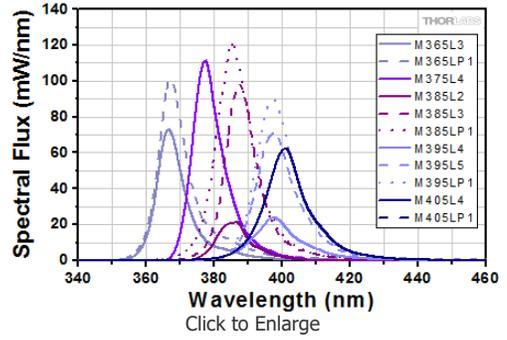
Visible LED Spectra Scaled to Min Power
