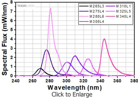
UV LED Spectra Scaled to Min Power
